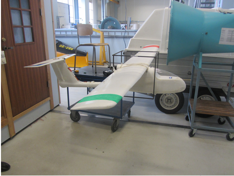
Figure 7: HINUAV-1 during trifilar inertia experiment, the Z-axis is being measured.
