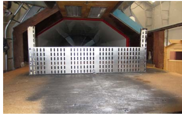
Fig. 2. Physical wind tunnel experiment setup.
