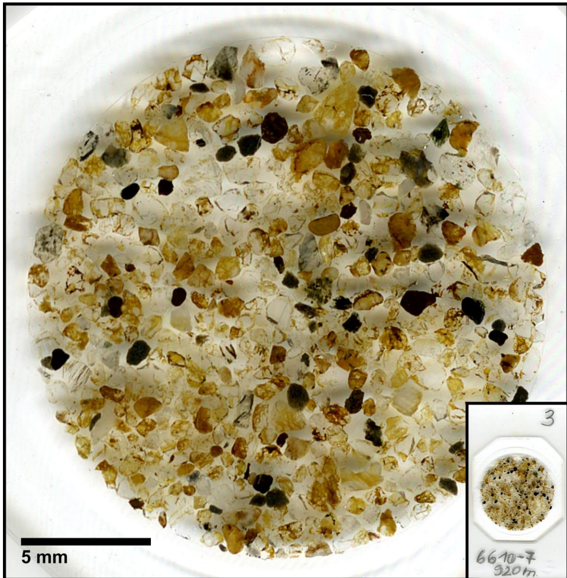
Figure 26: Exemplary true-colour scan of an offshore sample (well 6610/7-1, 920 m) with siliciclastic sand of the grain size fraction > 0.5 mm embedded in epoxy resin. Inlet in bottom right-hand corner displays the actual size of the slide.
