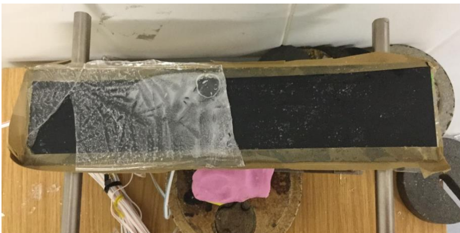
Figure 13: Failure in a 5 mm ice sample
