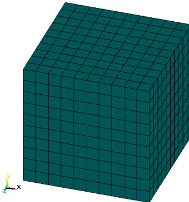
Figure 6: ANSYS® Multiphysics Mesh of 3D space
