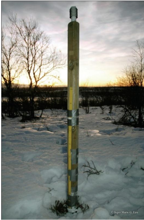
Figure 3: Temperature Monitoring Solutions Thermochrons on a pole in a winter pasture area in Kautokeino, des. 2008.
