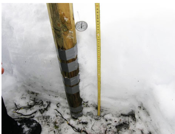
Fig. 8.12 NASA thermochrons at Saami snow station (photo by I.M.G. Eira)
