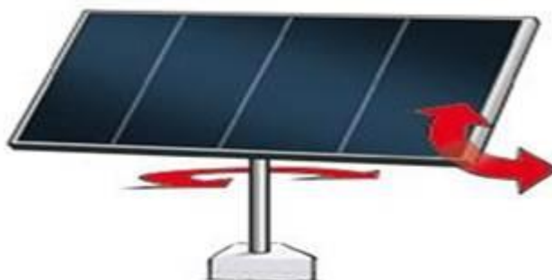
Figure 2.5.2 Tip-Tilt Dual-Axis Solar Tracker [27]
