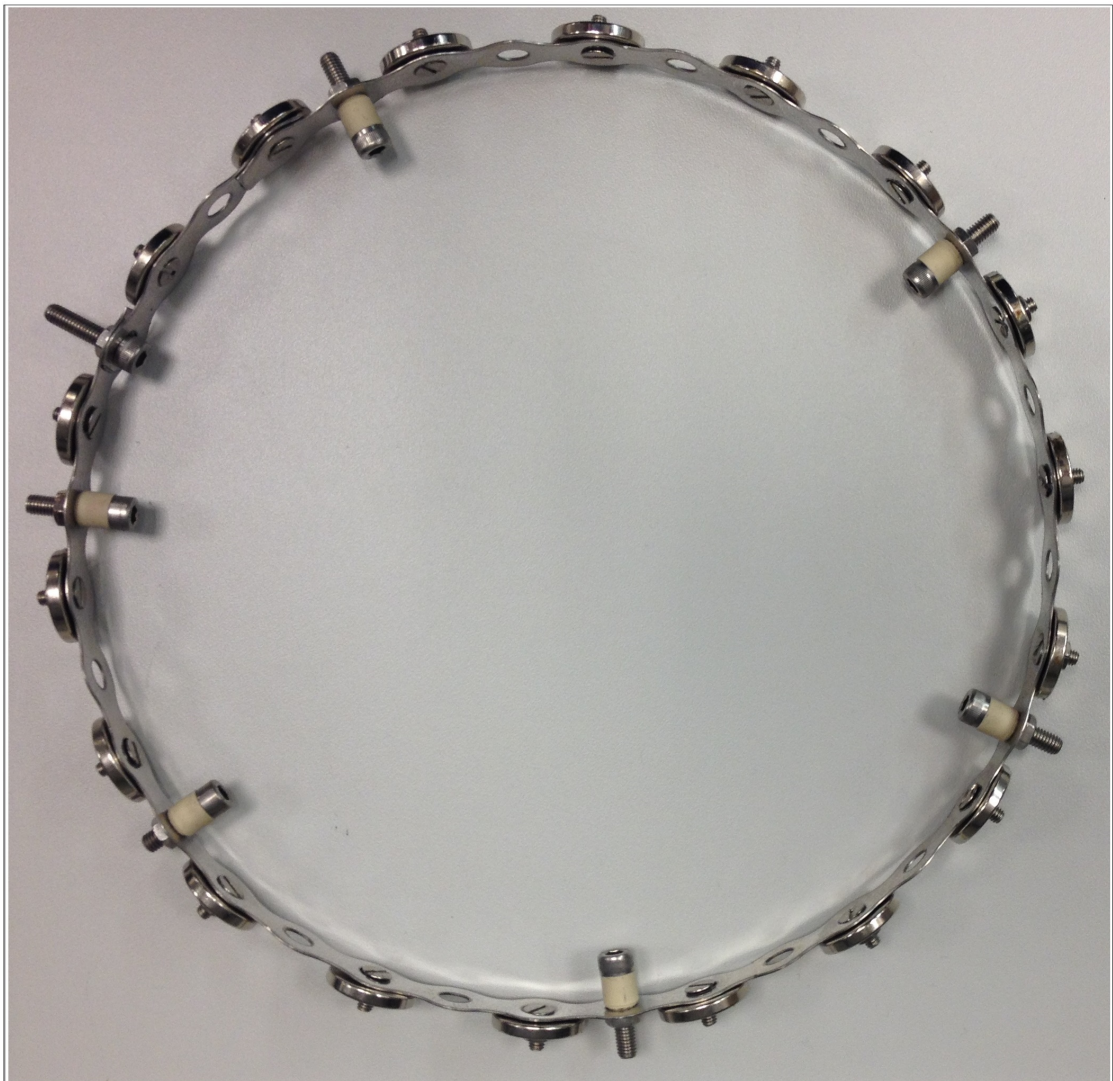
Figure 3.5: The band with the magnets which creates a cusp field.
