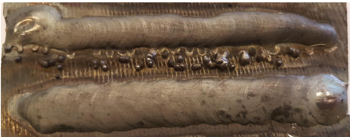
Figure 29: Welding with feeder out of alinement with the arc
