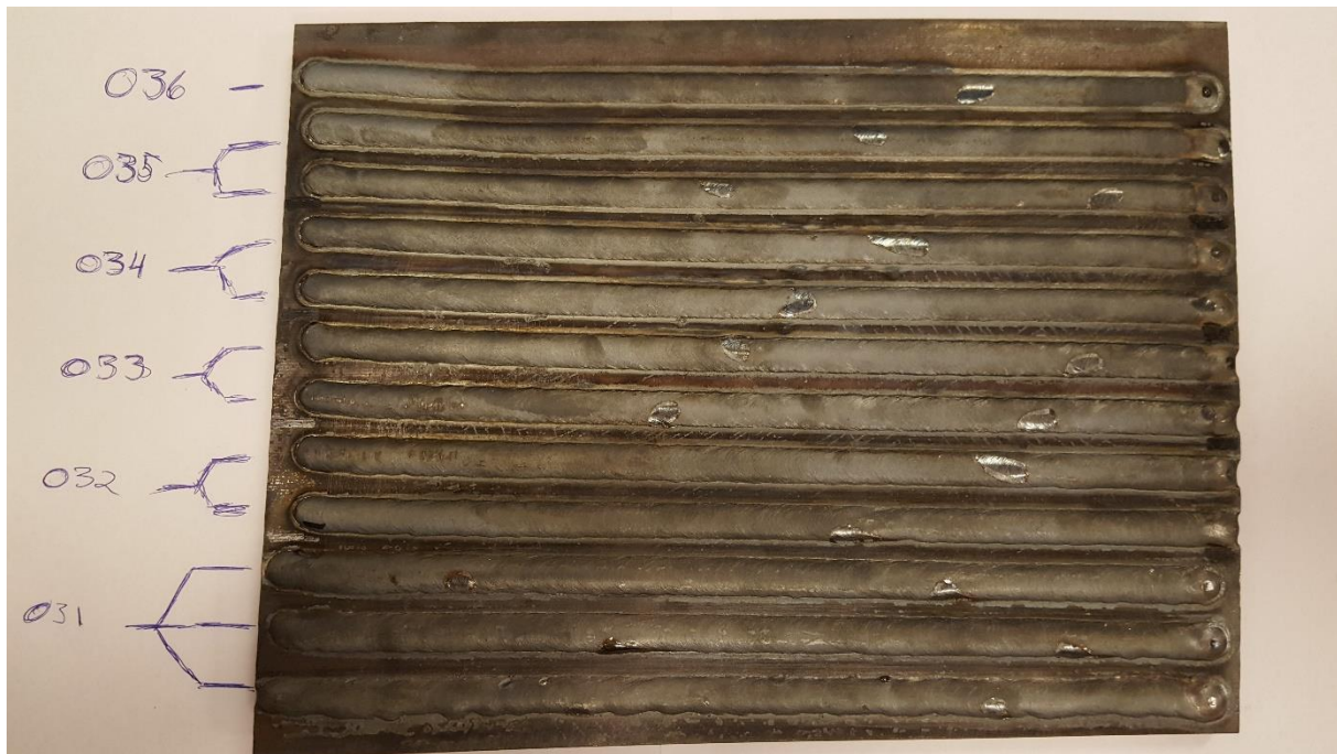
Figure 21: Test weld 031 - 036, speed test 180 - 300 mm/min
