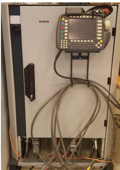
Figure 3: KUKA KR C 2 controller with teach pendant
