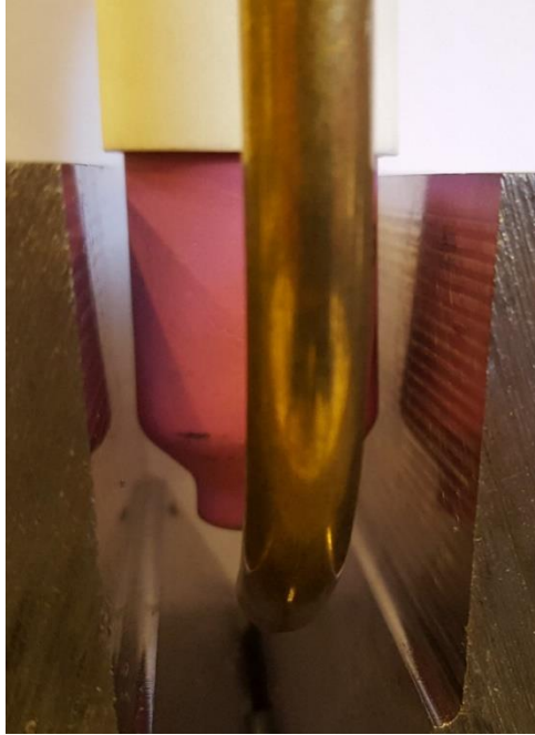
Figure 35: Weld groove too small for the torch
