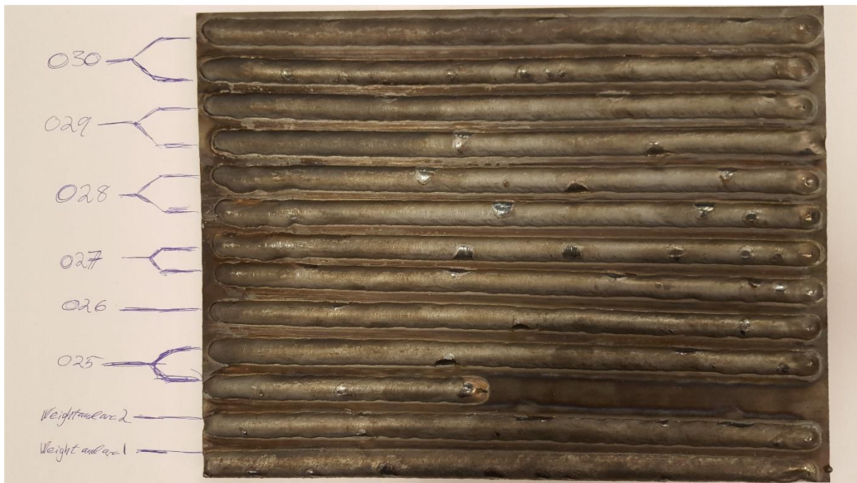
Figure 20: Test weld 025 - 030, feed test 300 A
