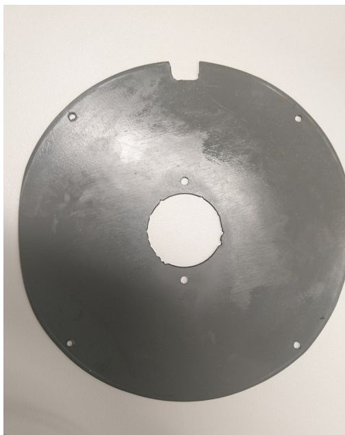
Figure 3.11: The PVC insulation separating the grids in the plasma source with a melted inner rim.
