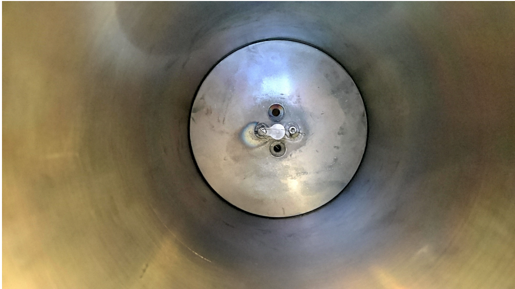
Figure 3.2: View inside the anode cylinder and plasma source, where the cathode filament is stretched horizontally across the diffuser disc in the middle.
