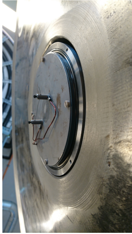
Figure 3.6: Plasma source installed in SSC. View of neutralizing filament and outer grid
