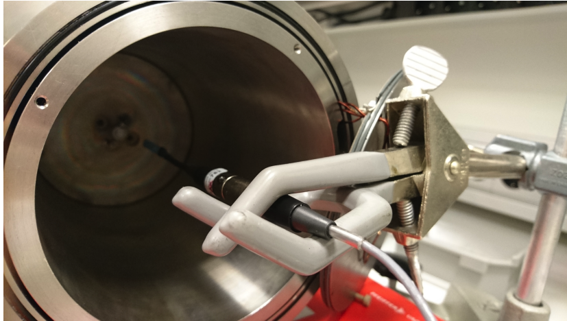
Figure 3.3: The axial probe of a gaussmeter is installed on a mount to test the magnetic field strength, produced by the solenoid, inside the plasma source.
