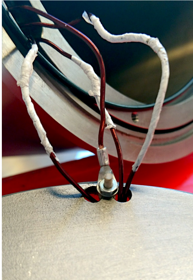
Figure 3.13: The inner grid disc with the connecting wire screwed on. Also seen passing through are the two wires for the neutralizing filament and one for the outer grid.
