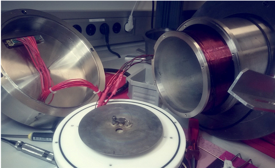
Figure 3.1: The disassembled plasma source as the cathode filament is being changed
