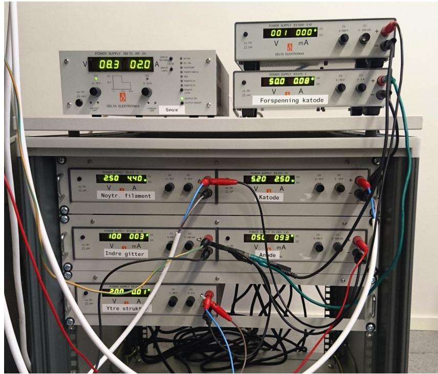
Figure 3.8: The setup of the different power sources needed to run the plasma chamber (see table 3.1 for details).
