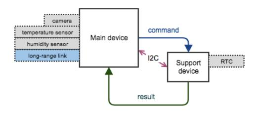
Figure 3.2: The observation unit's main components.
