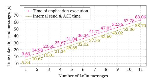
module preparation times are roughly constant, independent of the number of messages sent and oscillate around 4.35 second (+- 0.02s).
