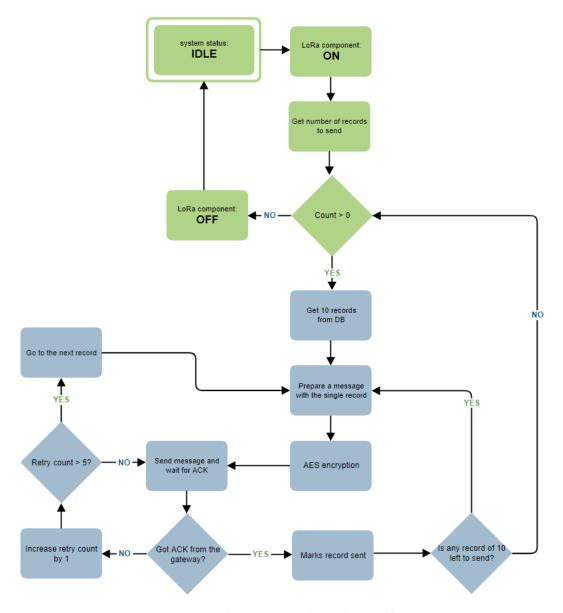
Figure 4.3: The LoRa module application flow.
