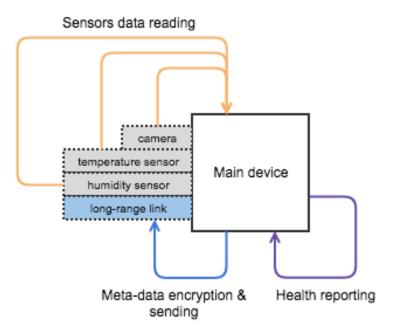
Figure 3.3: The main device's functionality.
