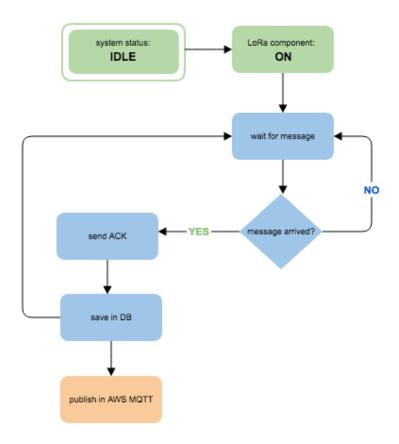
Figure 4.5: Gateway applications flow.
