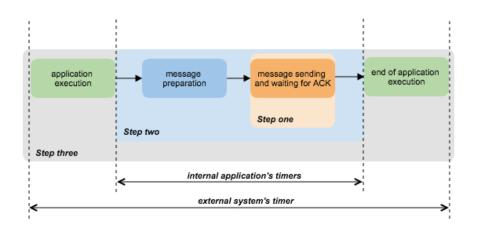
Figure 5.1: Time measuring steps in LoRa Bandwidth scenario.
