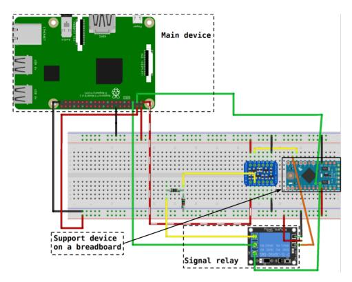
Figure 4.4: Connections between Observation unit's devices.
