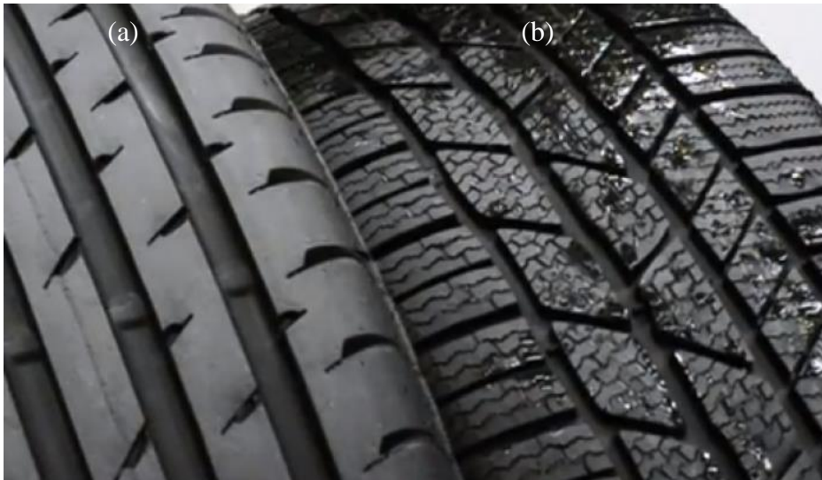
Figure 4: Comparison of summer tire (a) vs winter tire (b). [12]
