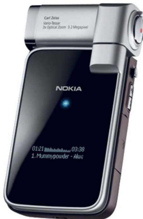
Figure 3: Nokia N93 with 3,2 megapixel camera, Mp3 player and WLAN interface.
