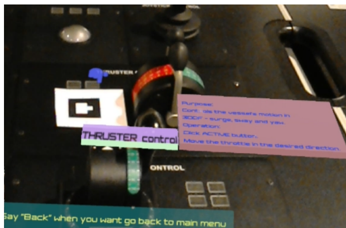
Fig. 4.15 Tracking result from Thruster control button on the steering panel. Hand shape can move up and down to point the button.
