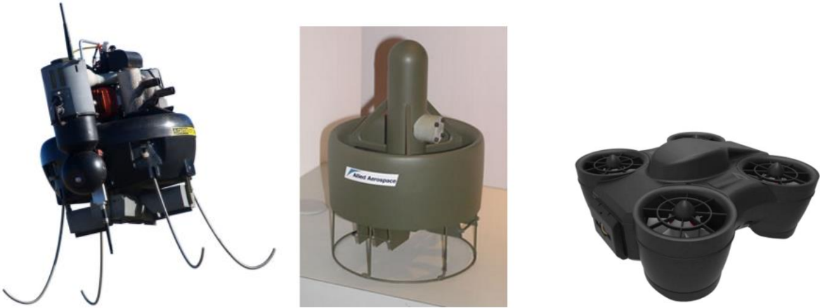
Figur 5. T-Hawk, iSTAR and the Nano Tornado ducted fan drones (Honeywell, 2009) (Defense update, 2017) (Indiegogo, 2017).
