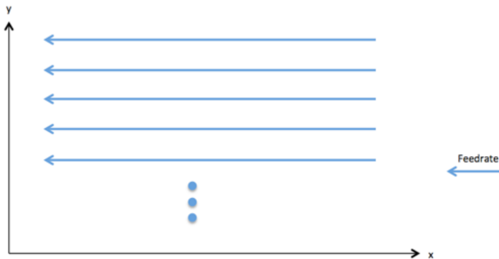
Figure 33 – Profile milling illustration of linear path only optimization solution (PM module)
