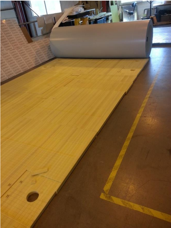
Figure 1 - Core configuration with a roll of aluminum facing in the background.
