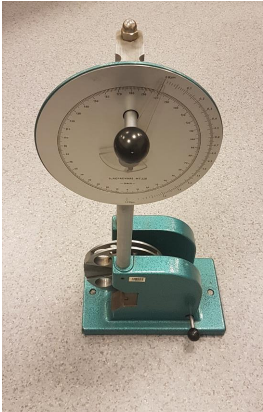
Figure 25 – The Charpy pendulum used in this project
