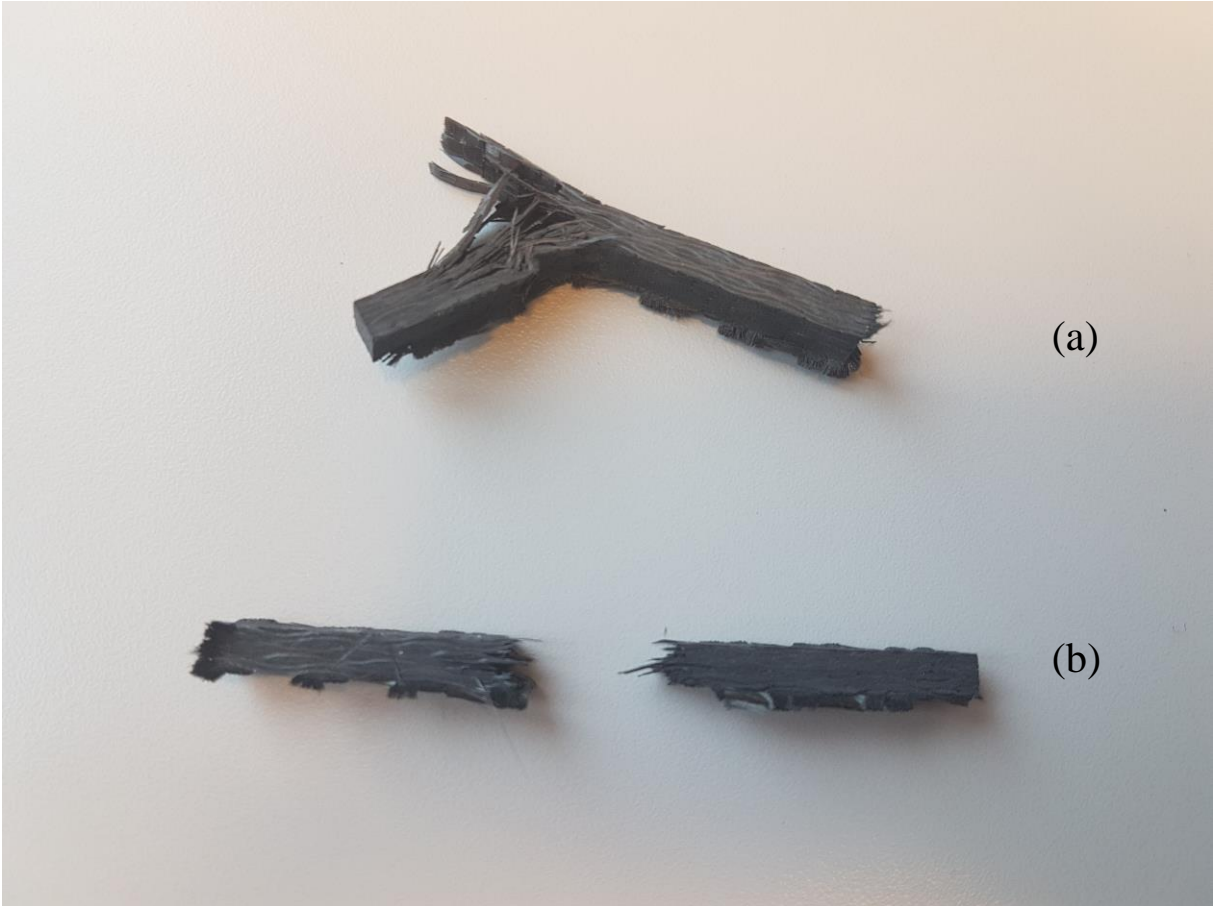
Figure 39 – A visual display of the qualitative results of the Charpy test
