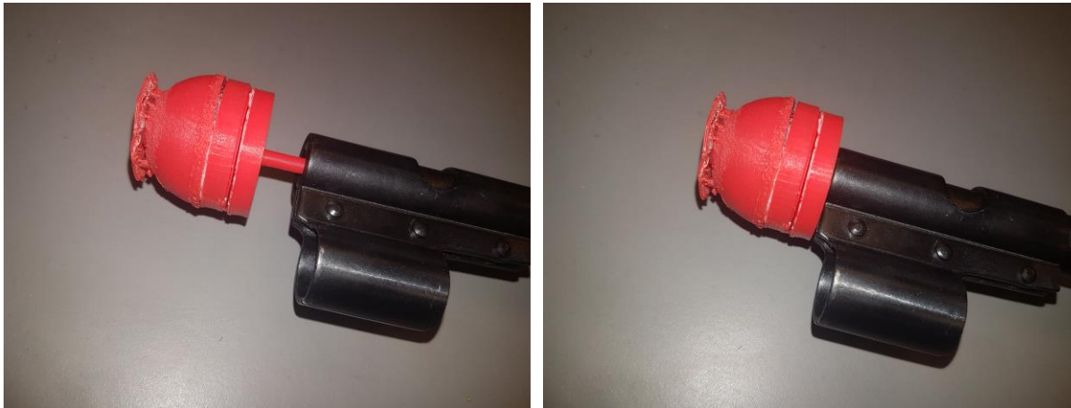
Figure 24 – The device for shooting ice on the CFRP test pieces, attached to the air gun.
