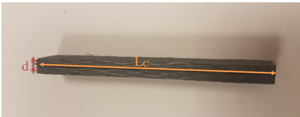
Figure 4 – The span-to-thickness ratio ( L_C/d ) of a test piece of CFRP.
