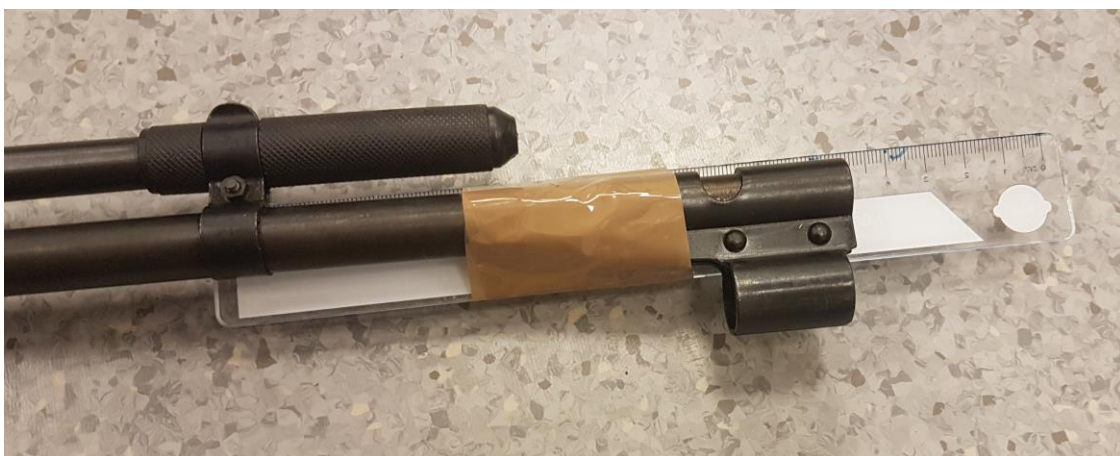
Figure 16 – To shoot at exact 60 mm distance from the test pieces, a ruler was attached to the barrel of the gun.
