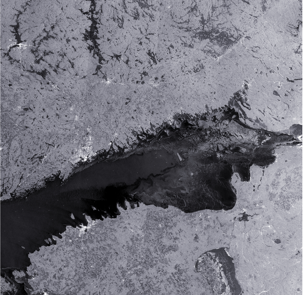
Figure 3: SAR image of the Gulf of Finland the 9th of June 2017 at 10 am, captured by Copernicus Sentinel-1B. Ships are identified as bright dots, sometimes shaped like stars because of their strong RCS. Photo:ESA
