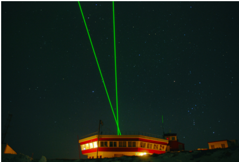
Figure 4: Arctic Lidar Observatory for Middle Atmosphere Research (ALOMAR), located in Andenes, Norway. The green laser beams are the RMR lidar. Photo by Trond Abrahamsen, from Andøya Space Center website[11].
