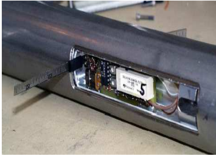
Figure 2.8: Faraday probe. Credit: [22]
