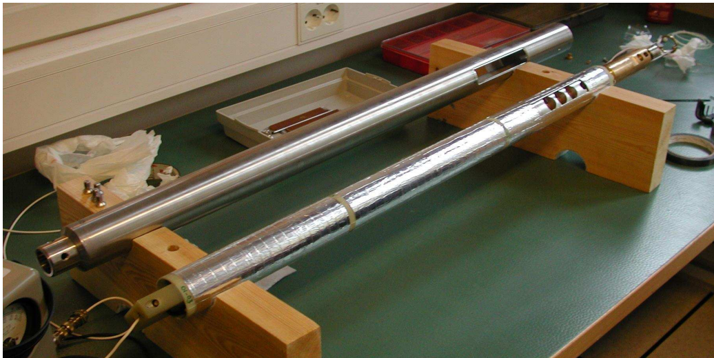
Figure 2.10: Outer hull and payload with heat insulation. Credit: [22]
