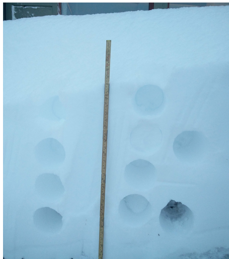
Figure 10.1: Photograph of the snow profile at 06/12, with round density profile cuts shown.
