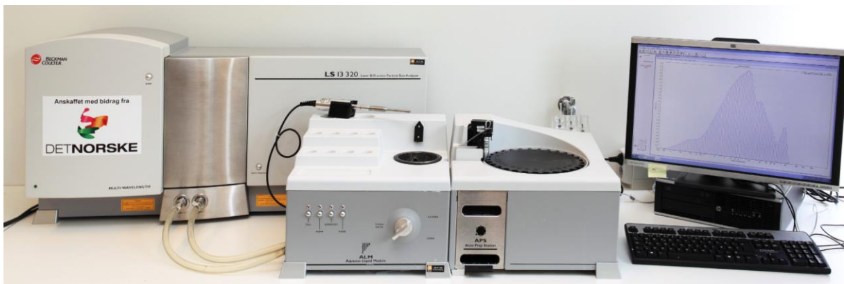
Figure 35 Beckman Coulter LS 13 320 Multi-Wavelength Laser Diffraction Particle Size Analyzer in the laboratory at the Institute for Geoscience, UIT. Photo by (T. Dahl et al.).
