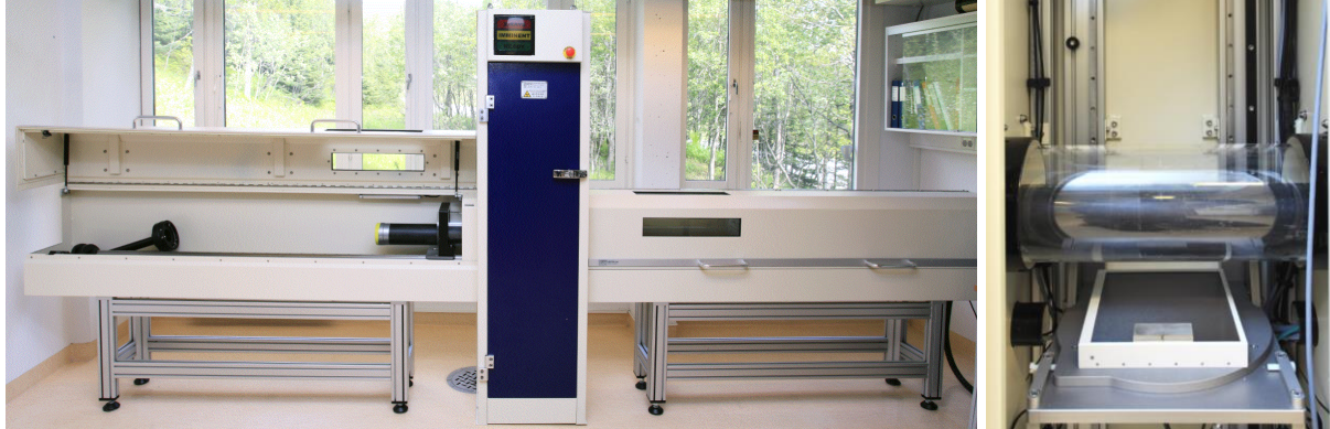
Figure 33 The Geotek MSCL X-ray Computed Tomographic imaging machine laboratory at the Institute for Geoscience, UIT. Photo by (T. Dahl et al.).
