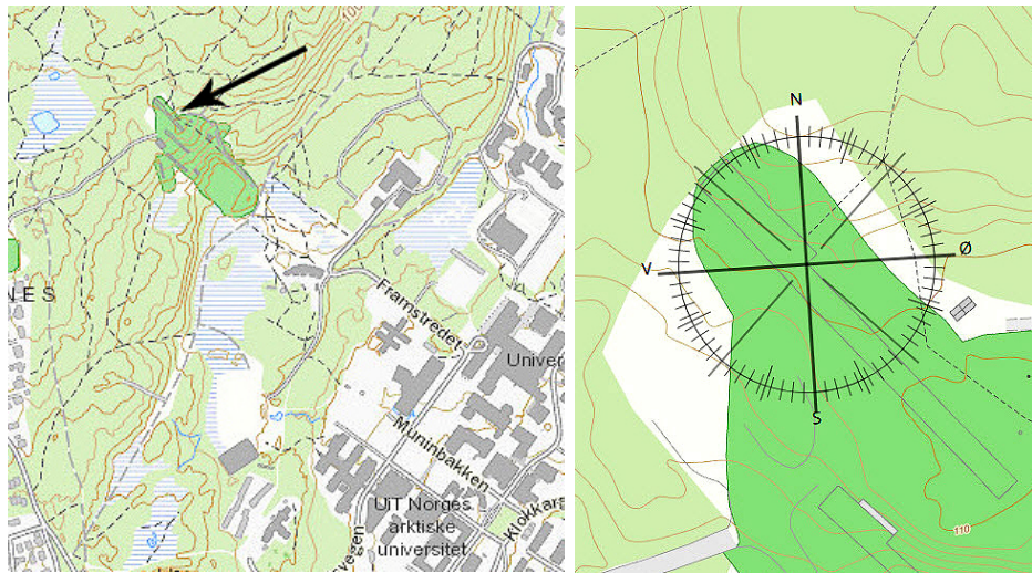
Figure 4.18: Map of the area where the ski-jump is positioned. The buildings in the bottom right corner of the left image belong to the University of Tromsø. The map on the right shows a compass centred in the position of the anemometer. The angle between magnetic north and the railing used to align the anemometer is shown to be 50 \pm 2 degrees. Maps taken from [2].
