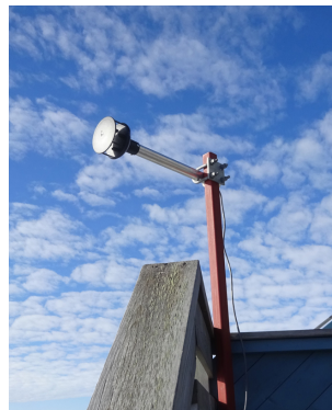
Figure 4.19: Anemometer on ski jump measuring vertical wind. [Photo: Simma]
