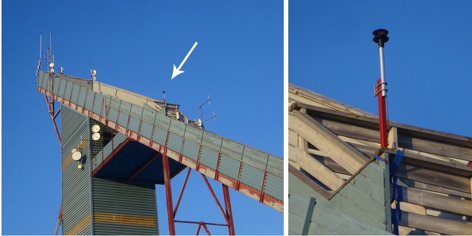
Figure 4.17: The WindSonic anemometer mounted on the ski jump tower to measure horizontal wind. [Photos: Simma]
