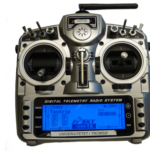
Figure 2.7: Remote control: The left stick controls the throttle and yaw angle while the right stick controls pitch and roll angles. [Photo: Simma]
