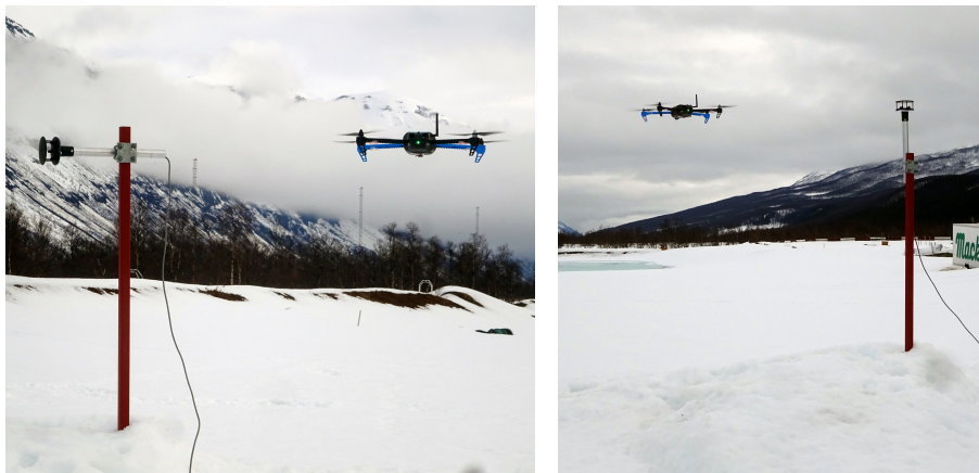
Figure 4.22: Ramfjordmoen test flight site with two different anemometer configurations and the quadrotor flying close to it. [Photos: Simma]
