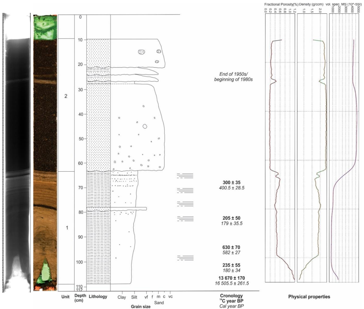
Fig. 124 Lithological log of core NL2 with x-ray image, photo of the core surface, lithological units, chronology and physical properties (fractional porosity, density and magnetic susceptibility)
