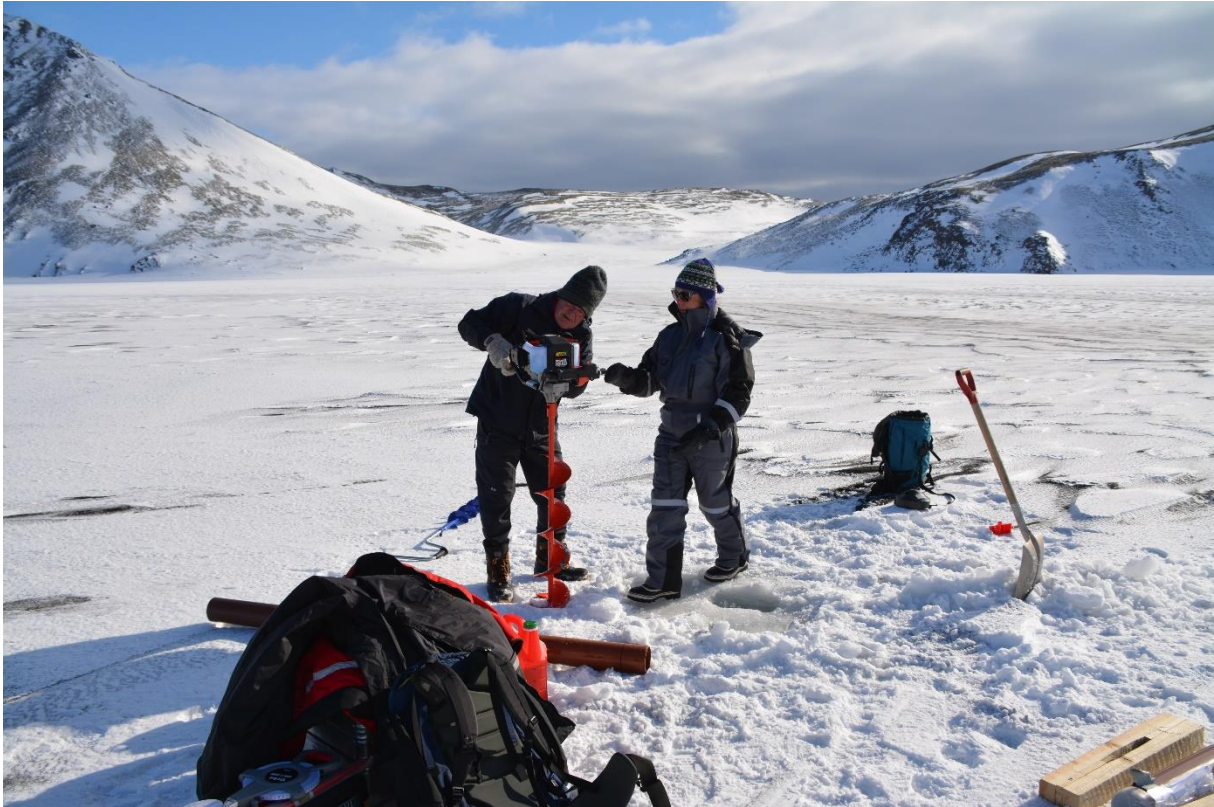
Fig. 13 Collecting of sediment cores from winter ice at Nordlaguna (photo: E. Larsen)
