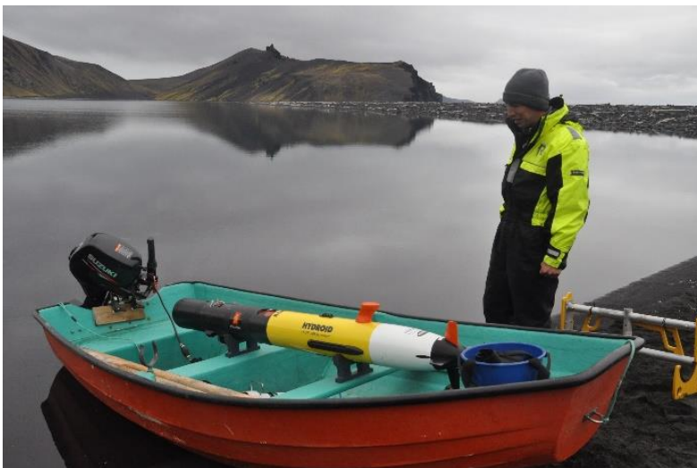
Fig. 14 Remotely Operated Vehicle (ROV) with Side Scanning Sonar (SSS) (photo: E. Larsen)
