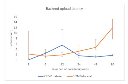
**Figure 6.2:** The average upload time in minutes for the two synthetic datasets, including the maximum and minimum upload time for each number of parallel uploads.
