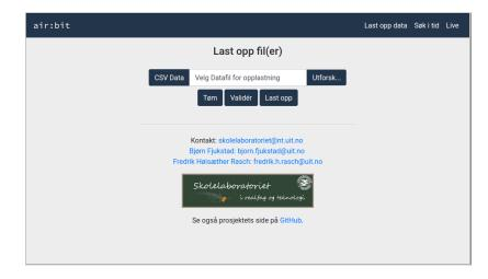
**Figure 4.2:** The air:bit web application provides a simple upload interface that also includes data format validation.
