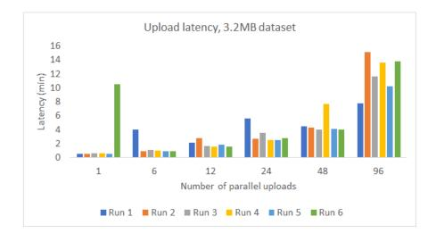
Figure 6.4: The upload time for each of the six benchmark runs for the 3.2MB dataset.
