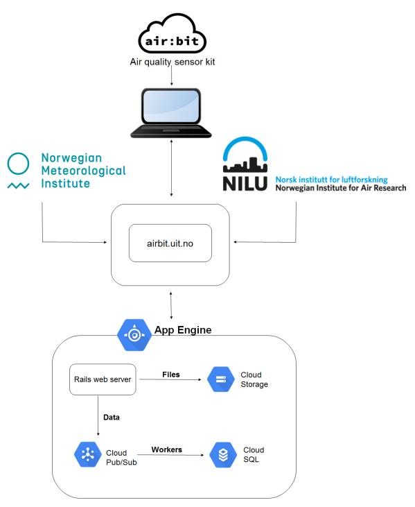
Figure 4.1: The air:platform design.
