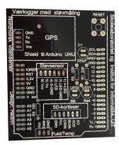
(b) The custom PCB Arduino shield.
