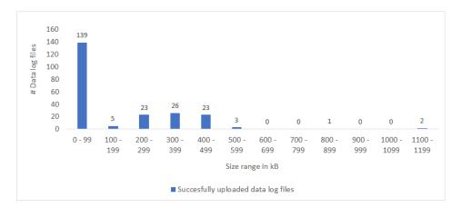
**Figure 6.1:** The size distribution of stored data log files in the backend database, for files uploaded from February through April 2018.
