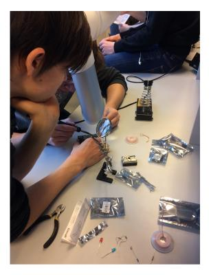
Figure 2: Students soldering different components of the air quality sensor kits to the custom PCB Arduino Shield.
