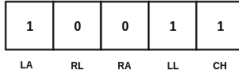
Figure 4.3: Example of 5 bit code corresponding to the sensor distribution that uses sensors on the left arm, left leg, and chest.
