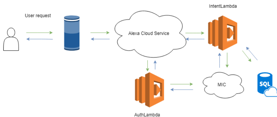
Figure 5.1: AlexaMIC architecture. All requests, except requests related to authentication originates from the Echo and are processed by the Intentlambda. Data from the local data store is fetched when required, and requests are dispatched at MIC. The AuthLambda handles authentication and re-authentication based on refresh tokens and the OAuth2 code grant flow.
