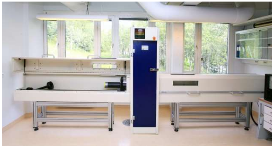
Figure 8: Geotek x-ray core imagine system at the University of Tromsø (uit.no, 2018. X-Ray instrument)
