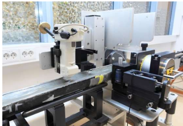
Figure 11: MSCL at the University of Tromsø (uit.no, 2018. MSCL with spectrophotometer)
