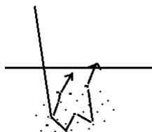
Figure 2.8: Illustration of volume scattering.
