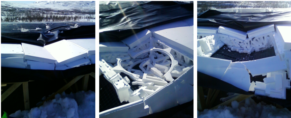
Figure E.10: Cell #11 of the test HBA tile. Left: The cover has been removed to show the fractured lid of Cell #11. Centre: the lid has been removed, showing the crushed internal structure. Right: the debris has been removed from Cell #11, showing the profile of Cell #10 behind it, as well as the sagged ground-plane and lower PVC bag.
