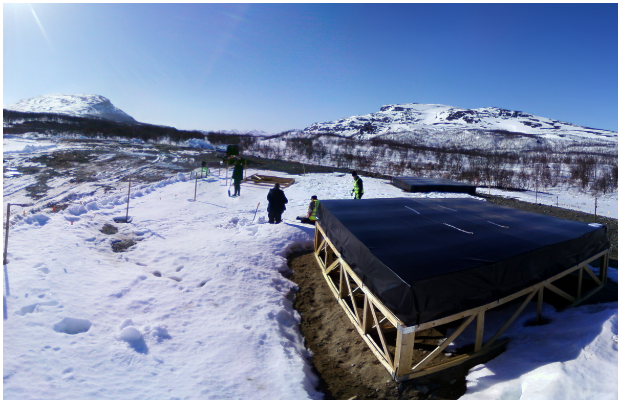
Figure E.7: Composite image taken on 10 May 2011 of the KAIRA site. The raised test tile is in the forward right of the image, with the ground-placed tile beyond it. The mountains of Saana and Pikku-Malla are in the background (left and right, respectively).
