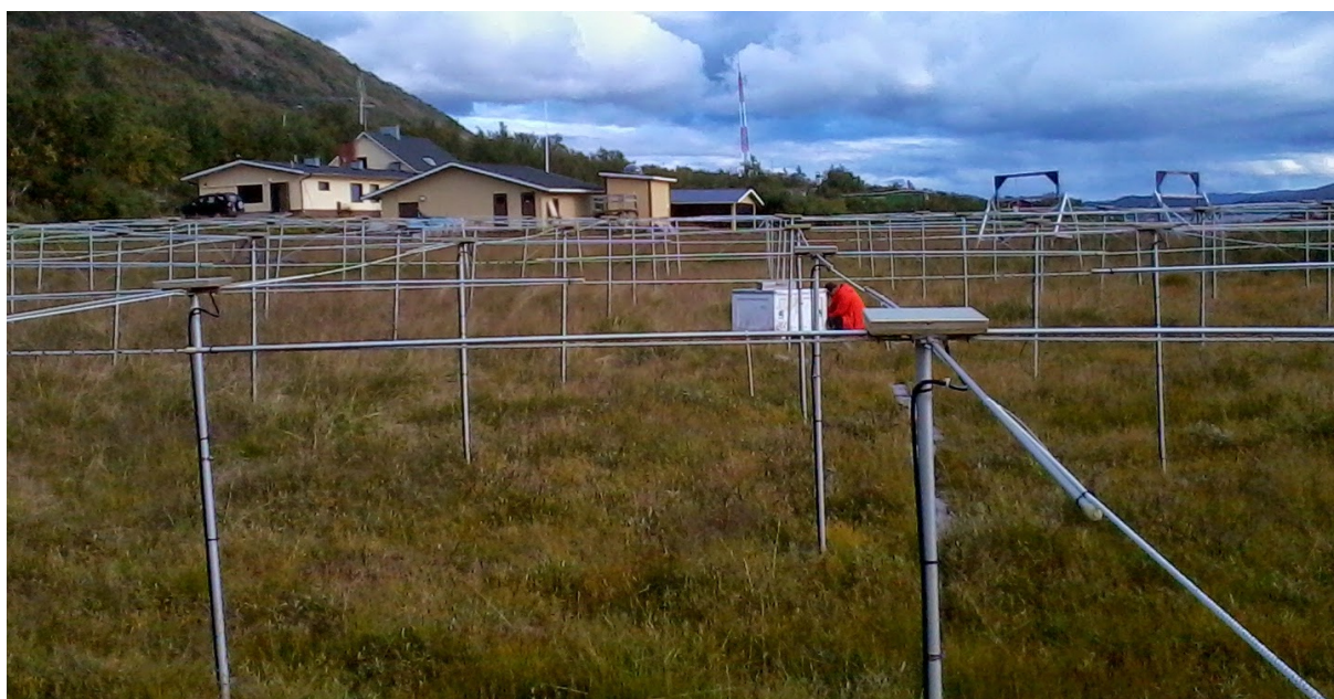
Figure 5.3: Southeast view across part of the dipole antenna matrix of the IRIS instrument. The building with the singularly-sloped roof has the FMI optical all-sky camera. The mountain in the left background is Saana.
