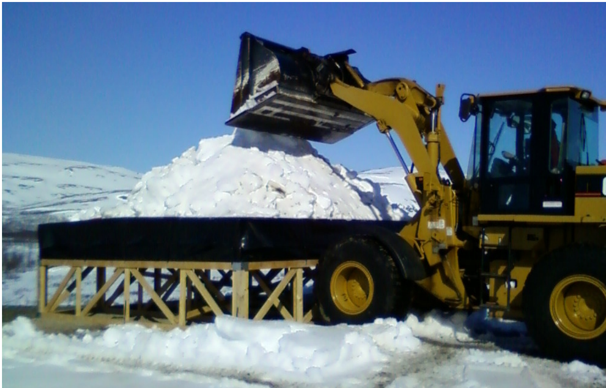
Figure E.9: Snow load #8 being deposited onto the raised winter test tile. Details of the snow loads are given in Table E.2.
