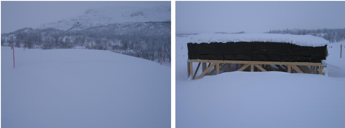
Figure E.6: Condition of the two winter test tiles on 18 February 2011 with the snow-buried ground tile (left) and raised tile and frameset (right). Compare with Figure E.5.
