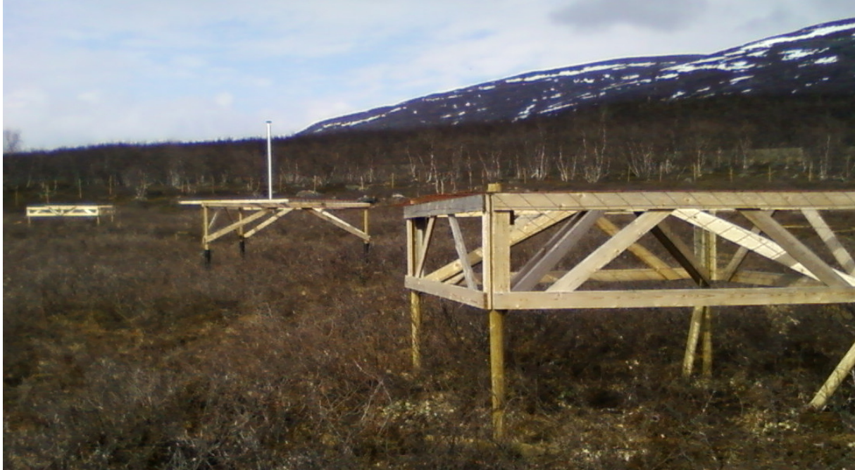
Figure E.39: The three test platforms in the lower field at the KAIRA site. All three are fitted with the RF ground plane, but only the centre platform has the LBA aerial erected at the time the photographs was taken.
