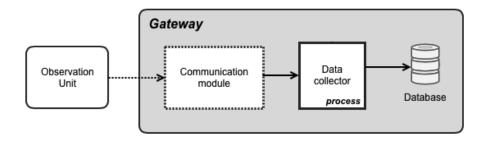
Figure 3: The Gateway software architecture.
