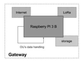
Figure 6: The Gateway prototype.
