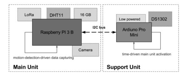
Figure 5: The Observation Unit prototype.
