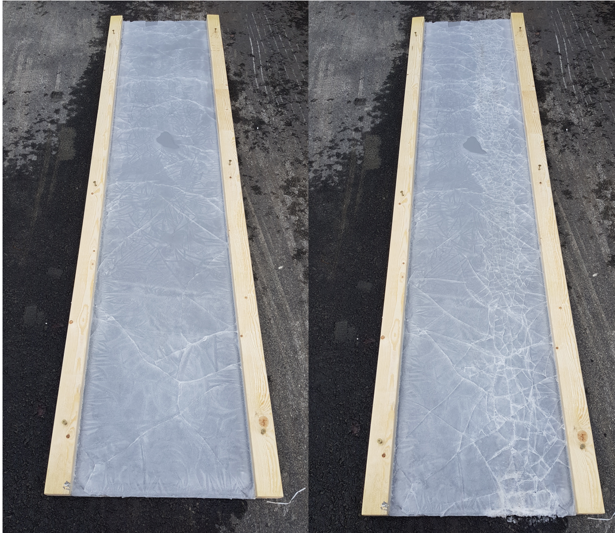
Figure 25: Before (left) and after (right) driving over anti-seepage polyurethane board
