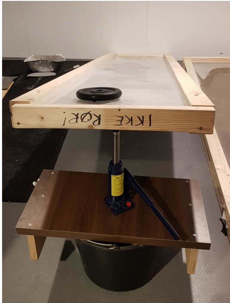
Figure 16: Setup for sliding friction testing with ice
