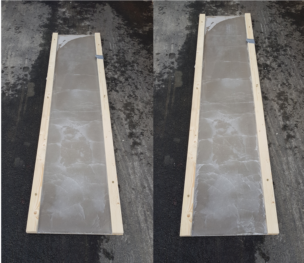
Figure 24: Before (left) and after (right) driving over concrete board
