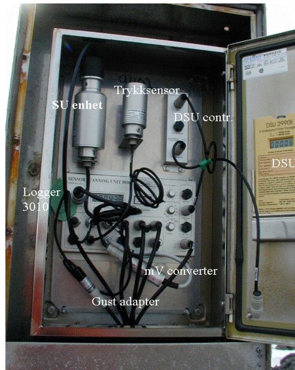
Figure 10: Hardware layout of the Norwegian Polar Automatic station
