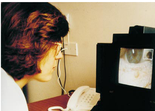
Fig. 4: Videoconferencing unit in use. A small digital camera, seen mounted on the top of the unit. (Source: Eedy et al. 2001)
