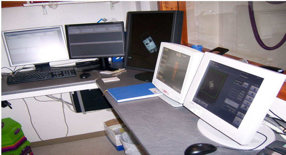
Fig. 17: (From right hand to left hand): Mobile set image shown in Computer (Com)-1, Com-2 enlarges the image; Com-3 shows enlarged image; Com-4 and Com-5 for email message exchange between nurse and specialist or radiologist. When nurse confirms that image quality is OK, then S/he can send the given image to specialist (dermatologist) or radiology dept. of UNN via Com-1.
