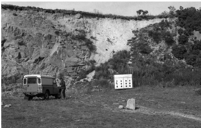
Figure 11 Gruss pocket at Cairngall Quarry, Mintlaw, Buchan, developed in medium-grained biotite granite below a thin till cover. Gruss
