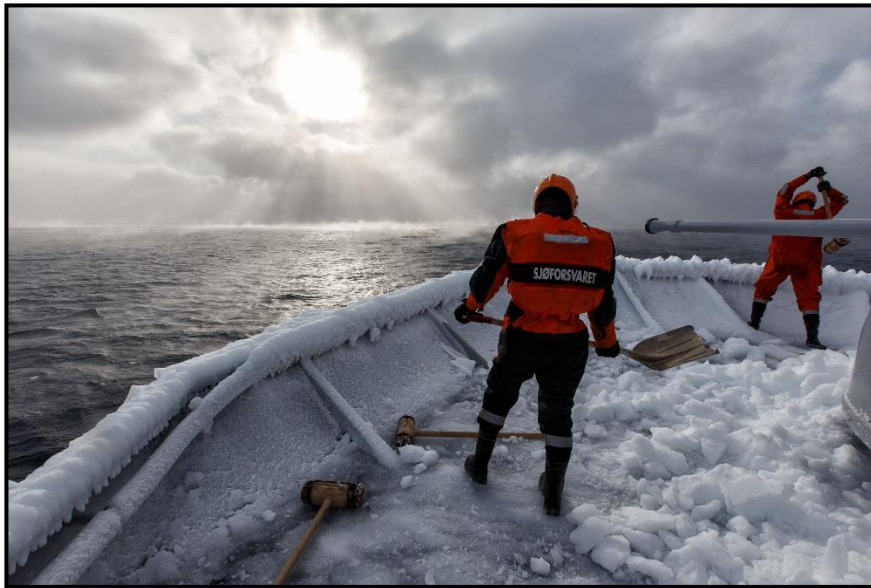
Figure 2: Ice accretion on a ship (Photo credit: Norwegian Coast Guard/Håkon Kjølmoen)
