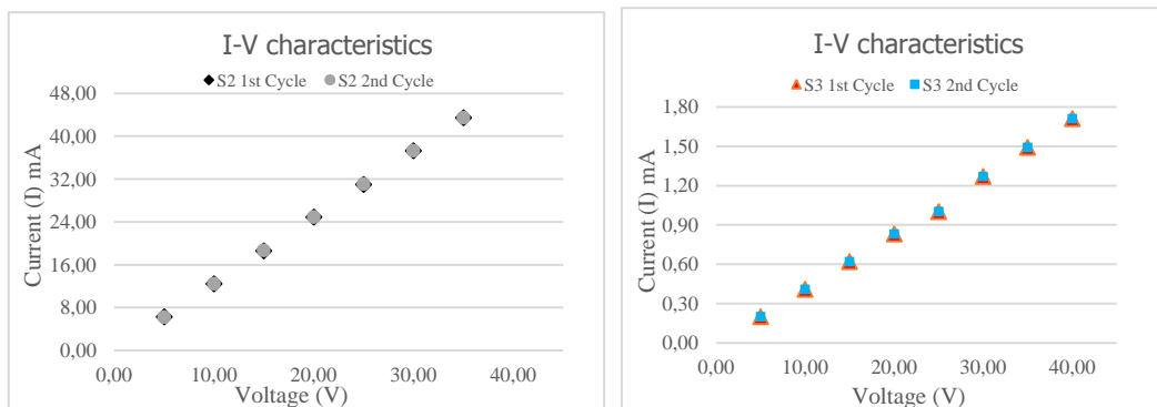
Figure 18: I-V characteristics of R2R CNT coated samples (S2 and S3) in Figure 3 of Paper IV
