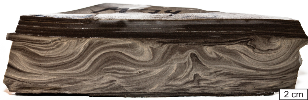
Fig. 3.20: Convolute lamination situated between two beds of planar laminated siltstone. The upper part of the convoluted unit was eroded prior to the deposition of the overlying siltstone. Polished slab from 92.95 m above base.
