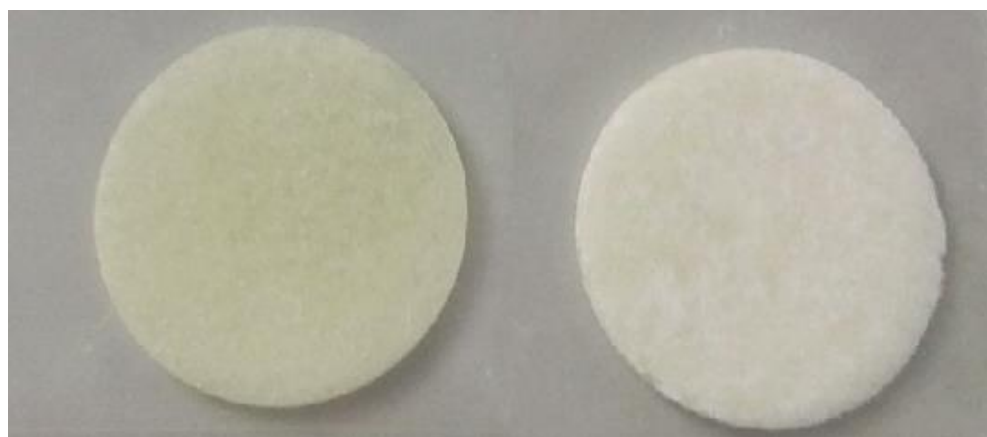
Figure 28 VCM-disks of CCX:Soluplus. 10% CCX (left) and 30% CCX (right). Prepared at 100°C from physical mixtures for temperature sweep analysis
