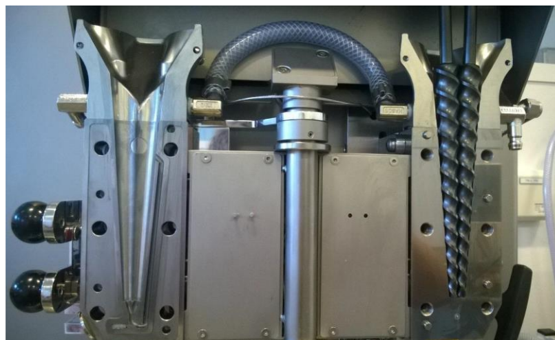
Figure 17 Laboratory scale extruder with a co-rotating twin-screw setup (DSM Xplore Micro Compounder)
