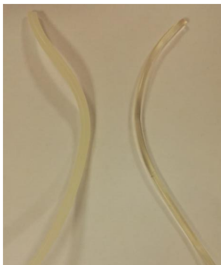
Figure 24 Comparison of extrudates of 50:50 CCX:Soluplus at different temperatures. 120°C with no recirculation (left) and 130°C with 5 minute recirculation in the extruder
