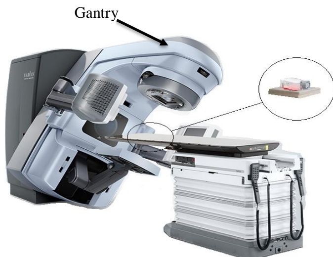
Figure 4.3: Varian clinical linear-accelerator: T-flask with CAFs were placed on top of tissue-equivalent plates (30 mm depth) with gantry position beneath the T-flask.
