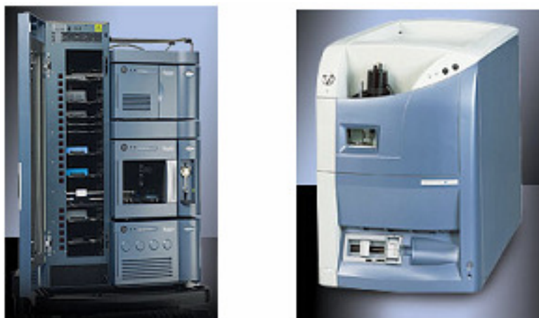
Figure 2 UPLC-MS/MS, Waters Acquity Quattro Premier XE system
