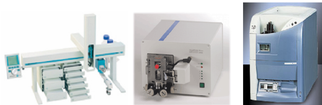
Figure 3 HPLC-MS/MS, CTC auto sampler, Rheos 2000 HPLC pump, Waters Quattro Premier XE
