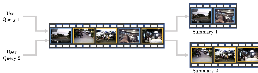
Figure 1. The illustration of the query-conditioned video summarization task. Given a user query, query-conditioned video summarization aims to predict a summary that is relevant to the query in a concise manner. Summary 1 and Summary 2 are two summarization results for the same video but for different user queries.
