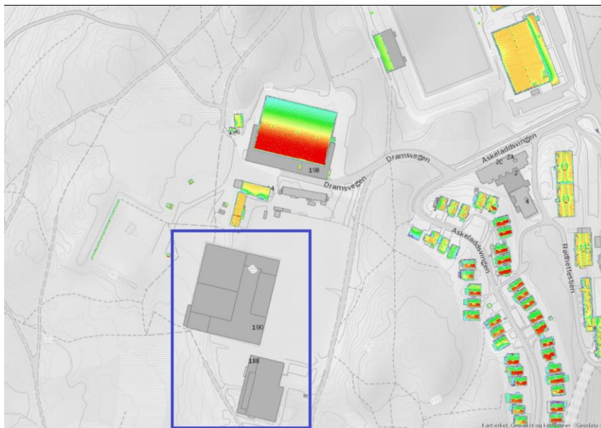
Figure 5-1: Tromsø skiing stadium, the new swimming pool is not a part of the solar map as the LiDAR dataset was created in 2014.
