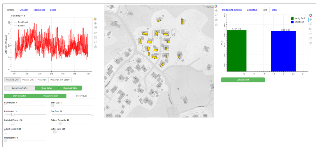
Figure 1. The FLEXNETT user panel showing time series for consumption and production on the left, the GIS panel in the middle where a selection of houses belonging to the same grid connection is investigated. Right a set of tabs can display aggregated power and cost data for the group and per building.
