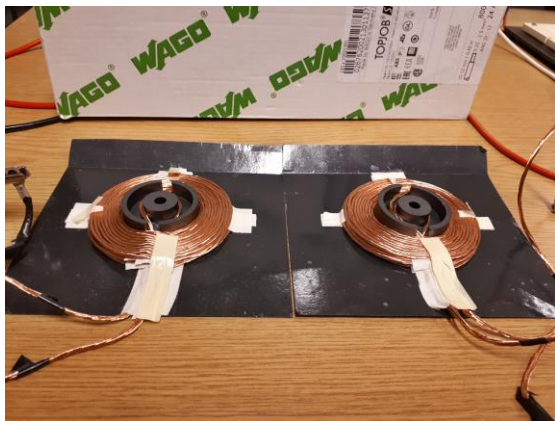
Figure 4.6: the transmitter (Tx) and receiver (Rx) Litz-wire coil I constructed
