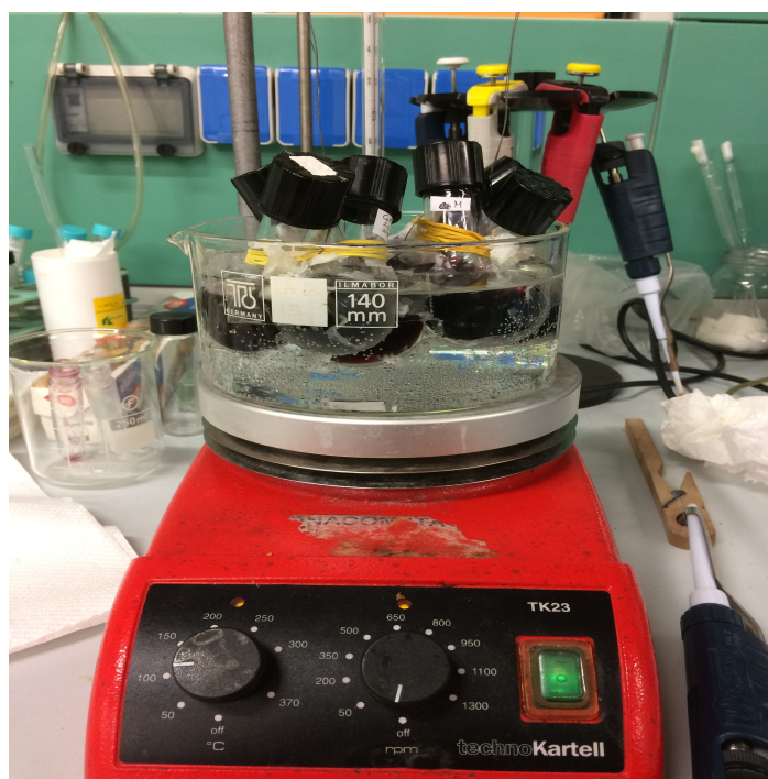
Figure 6 - Setup for the synthesis of nanoparticles at 70°C under vigorous magnetic stirring.
