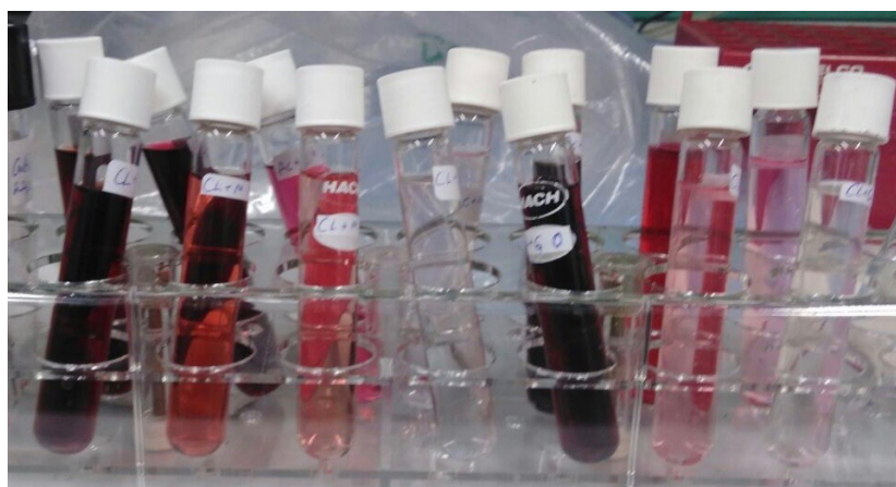
Figure 8 - Liquid decanted after each centrifugation step. From left to right: the 4 first tubes are \text{CuCl}_2 + myrtillus ; First decanting, second decanting (with citric acid sol.), third decanting (with citric acid sol.), fourth decanting with MilliQ water. The 3 next tubes are \text{CuCl}_2 + gaultherioides . First decanting, second decanting (citric acid sol.), third decanting (with citric acid sol.).
