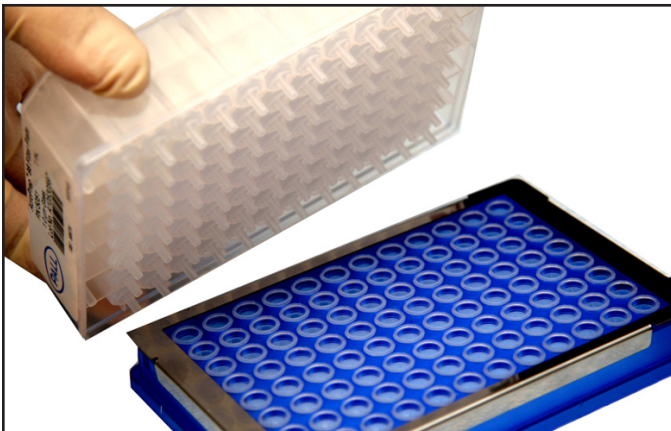
Positioning GF plate for elution step with a PALL collar
