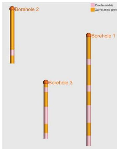
Figure 71: The different lithologies in the boreholes at Jettan.
