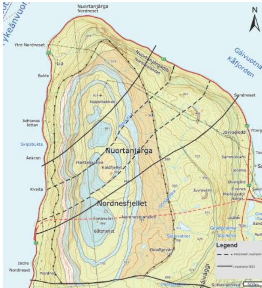
Figure 4: Lineaments and bedrock map at Nordnesfjellet. Modified from NGU (2019c).
