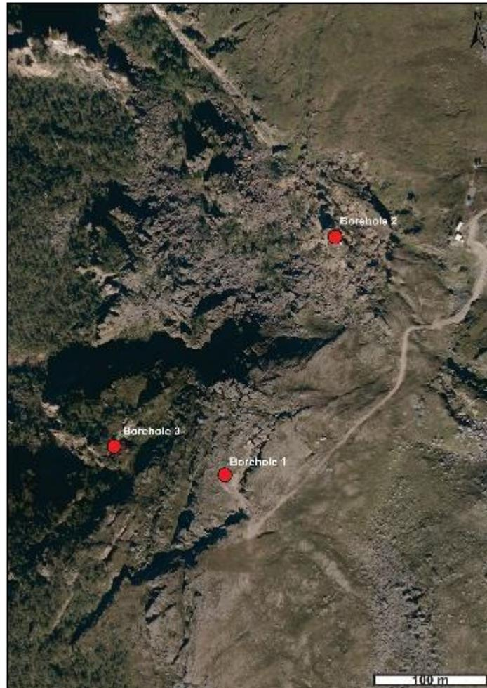
Figure 14: Location of boreholes at Jettan (Kartverket, 2016).
