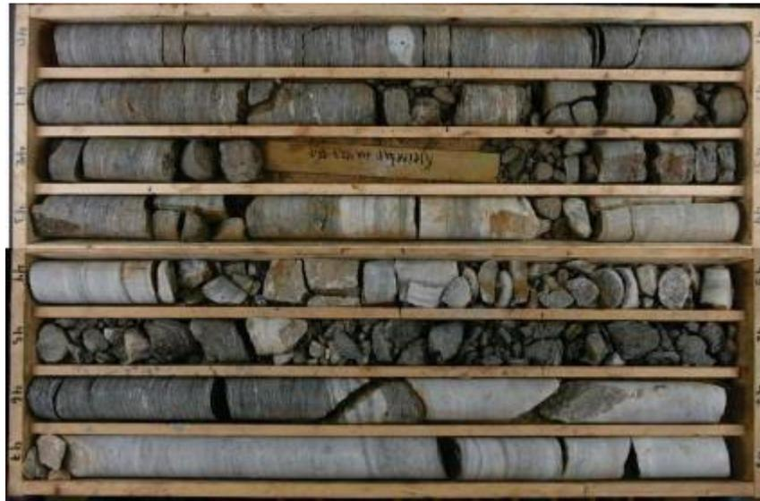
Figure 19: Main zone of crushed rock in borehole 3 at 42.3 to 46 m. Core loss is seen in the start of the zone and the rest is dominated by crushed rock. Modified by Ganerød (2014).
