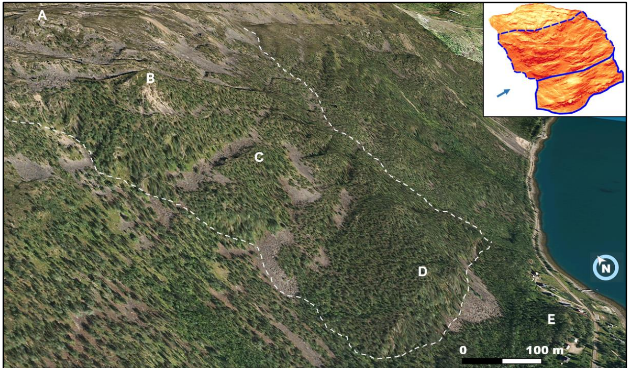
Figure 29: 3D-view of the deformation area Låvan (dashed line = limits of slope deformation): The small overview map depicts the direction of view (arrow) as well as the extents of the central (dashed, blue line) and frontal domain (full, blue line). A) The transition from the head domain to the steeper central domain is characterized by a system of minor scarps and counterscarps. B) Ridge belonging to the most prominent counterscarp (Figure 28). C) The rugged saw-tooth morphology of the upper central domain transitions into a more rounded stair-like morphology. D) A frontal lobe is only formed to a minor degree and ends abruptly at a cliff/scarp above the settlement Låvan (E) located on a flat coastal protrusion. The figure was created using ArcGIS Pro .
